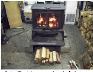
Allow the kindling to burn approximately 5 minutes. Flatten the coal bed with the included poker and load 10 to 15 pieces of medium size wood.
